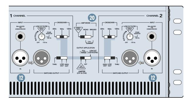
You can connect an unbalanced XLR cable to the M•2600, although this would be unusual — as unusual as an unbalanced XLR output. However, if you have an unbalanced XLR connection to make, refer to the "Connectors" section (*Appendix B*) at the back of this manual for more information.
